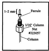
Figure 3.3. Capillary Column
