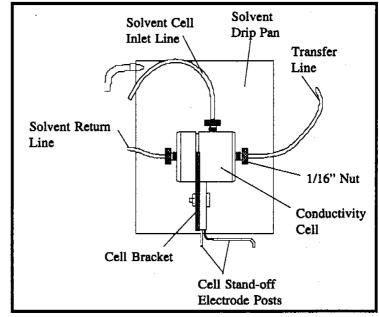
Figure 5.4. Conductivity Cell Assembly
