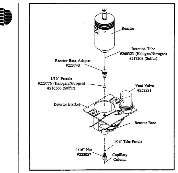
Figure 5.3. Reactor Base Assembly
