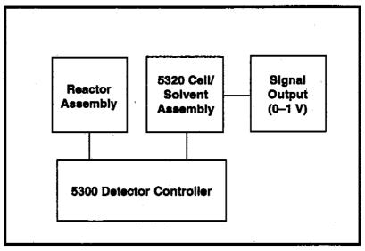
Figure 1.1. Model 5320 ELCD Principal Components
