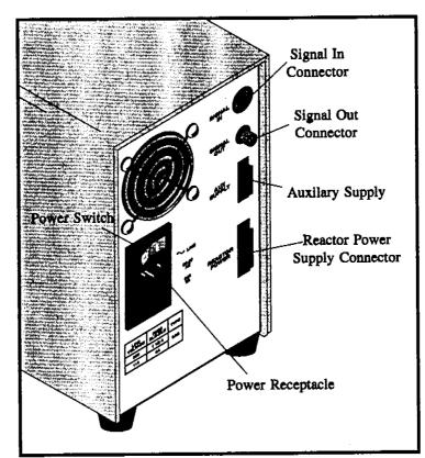
Figure 2.2. Detector Controller - Back View
