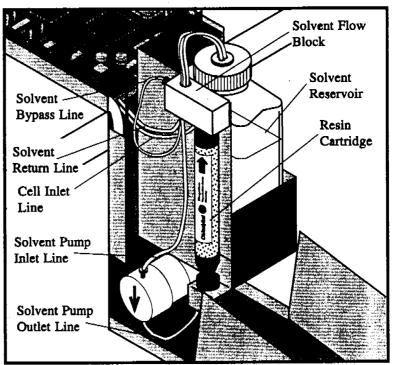
Figure 2.4. Cell/Solvent Assembly - Side View
